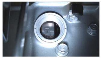
**AND (this is important)** the pulley marks align with the marks on the engine cover like here on LEFT side (seen from sitting on bike ... remember).
