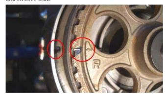
Mark this position on the central pulley and engine block.
