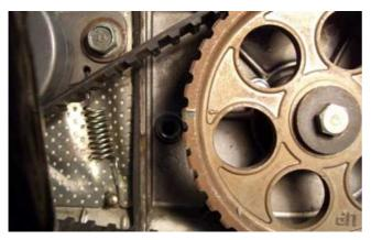
... This is, by the way, with the engine once more positioned at "T1".(\*) You then do the same trick with the tensioner (and the spanner as per Honda) locking it up after the spring has done its job".
