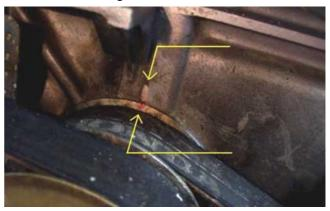
And check both cam pulley marks again.
