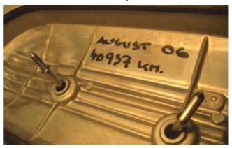
Check/re-adjust valve clearance and check/re-adjust ignition timing. New belts CAN move the ignition timing a much as a few degrees according to Randakk.
