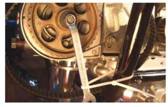
Do not use the spanner to turn the pulley. Use your hands ... then 'lock' it with the spanner. (Make <u>absolutely sure</u> you do not turn (release/loosen) the bolt).
