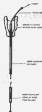
Oiling a control cable
