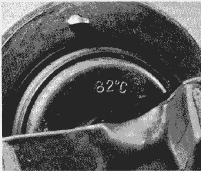
7.5 Note the vent hole in the thermostat case
