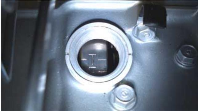
**AND (this is important)** the pulley marks align with the marks on the engine cover like here on LEFT side (seen from sitting on bike ... remember).
