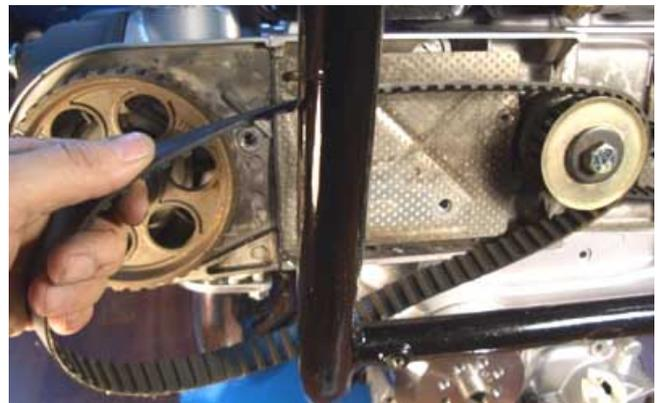
(\*) When you do that the right pulley (photo-left) will 'wander/turn' out of position when you remove the belt, as it is 'riding' on cam 'slope' (which is under the influence of the valve springs).
