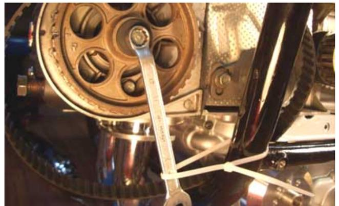
Do not use the spanner to turn the pulley. Use your hands ... then 'lock' it with the spanner. (Make absolutely sure you do not turn (release/loosen) the bolt).
