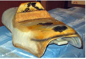
with contact cement as I was afraid that, with use, the foam would break down quickly. The contact cement dries and is not tacky after about an hour when applied to the foam. The last step here was to wrap the whole thing in clear plastic "Saran" wrap.
