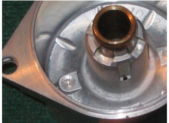
Cutoff valve cover has two channels to clean.
