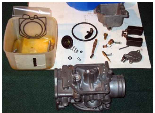
Take stock of the parts and arrange them for reassembly. Find all the necessary o-rings and new washers.
